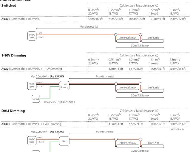
Note: This guide is produced from testing with KKDC approved power supplies or control gear.
