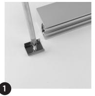
Fix clips with suitable screws (min. 3 clips per metre/40").
