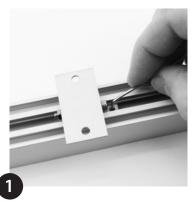
Slide bracket into required position and secure using grub screw.
